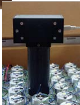
In-situ light output measurement
