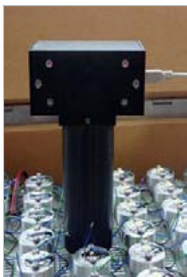
Fig. 5. LM80 test chamber, a) 60 devices and the liquid circulator for temperature control, in-situ measurement of the b) light output, c) thermal impedance (photos by courtesy of the University of Pannonia, Veszprém, Hungary).
