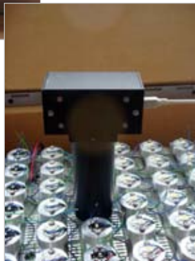
In-situ light output measurement
