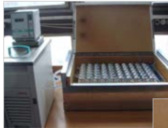
LM80 test chamber with all the LEDs assembled
