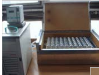
LM80 test chamber with all the LEDs assembled
