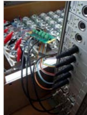
In-situ thermal transient measurement
